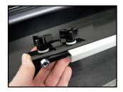
Install the "clip" of the stop without tightening the bolts. Make sure to well insert the clip. This should make a "click" and be strong once it is in good position.
