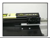
Adjust your cursor to allow the support to exceed approximately 1/2 inch or 1.2 cm of your blade when the cursor is at the end of the stop. This will enable efficient adjustment in the "zero" function of the stop. If your cursor goes no further than your blade, it will be impossible to get the zero point.
