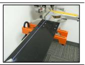
3 Draw a one (1) inch line in front of the line of the saw fence.
